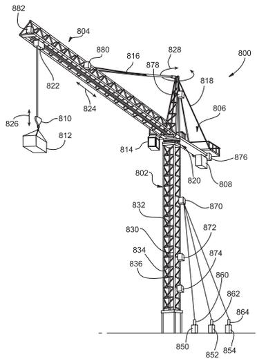
Figure 3. Measuring deflections of a tower crane.
