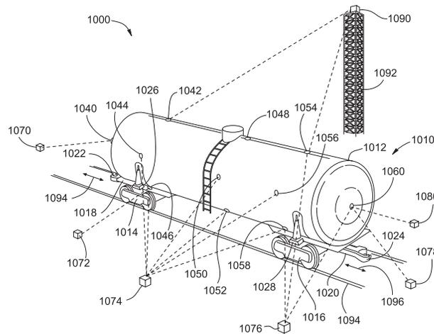
Figure 5. Measuring deformations of a railway tank car undergoing a pressure test.
