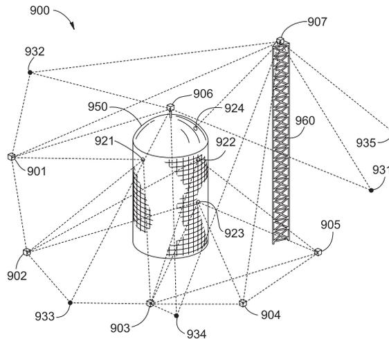
Figure 4. Measuring deformations of a nuclear power plant containment building undergoing a pressure test.
