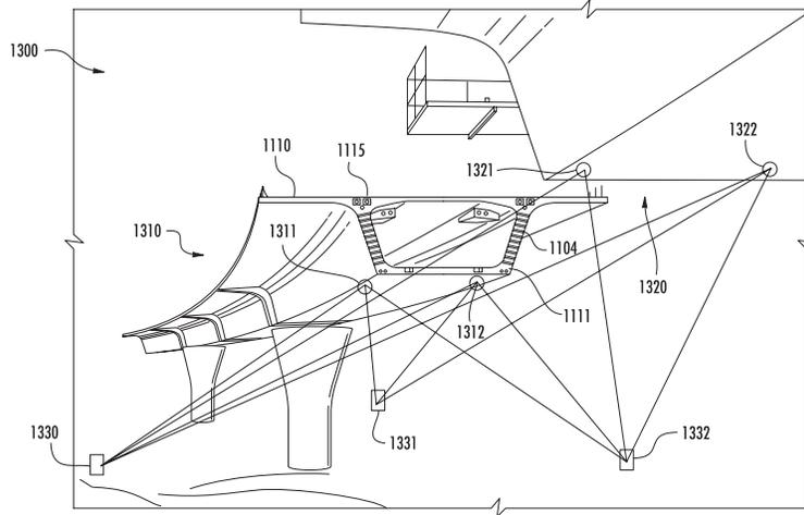
Figure 6. Measuring deformations of a bridge segment undergoing tensioning.
