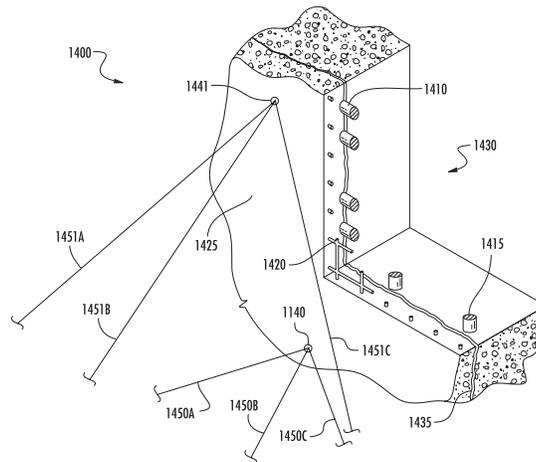
Figure 7. Measuring deformations of a nuclear power plant containment building undergoing detensioning.
